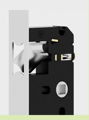
TO CHANGE DIRECTION OF LATCH LIFT LEVER, DEPRESS LATCH AND ROTATE 180 INSIDE OF GATE DIRECTION
