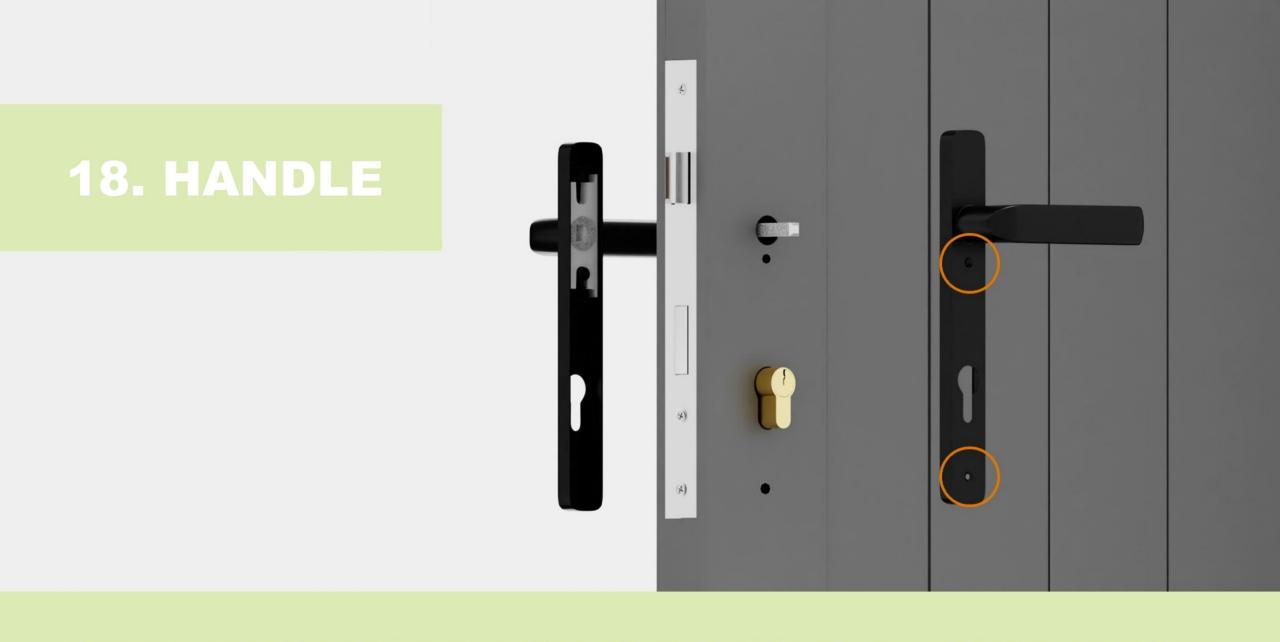
SET LH / RH HANDLE ENSURE FIXING HOLES TO INSIDE OF GATE
